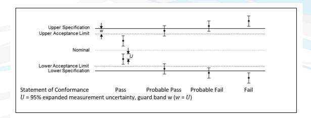
For a statement of conformity to be valid, any test conditions with non-measurable outputs, for example environmental conditions or equipment specifications, must conform to the requirements detailed within the test standard or specification.
